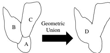
Fig. 2. Example of geometric union for catchments.
