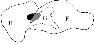
Fig. 4. Data-reuse Example –  $E$  and  $F$  are pre-defined regions. The black catchment is aggregated. Since the gray catchment flows into the black catchment, the gray catchment and its watershed, labeled  $G$ , must also be collected.
