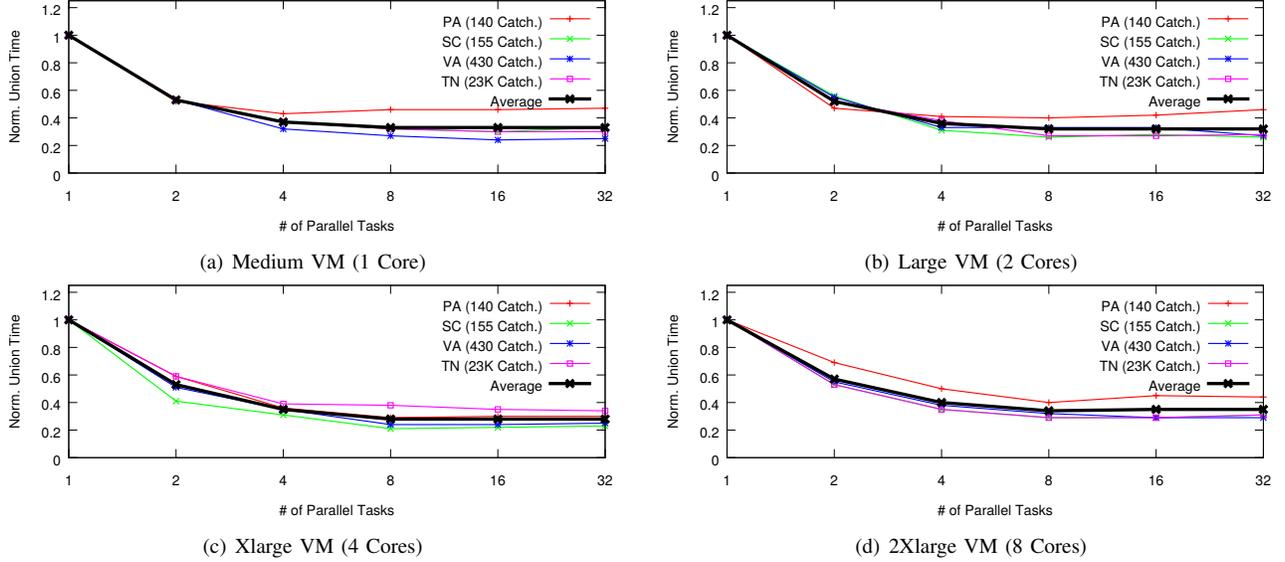
Fig. 7. Normalized geometric-union time of watershed delineation by parallel-union strategy on four types of VMs.
